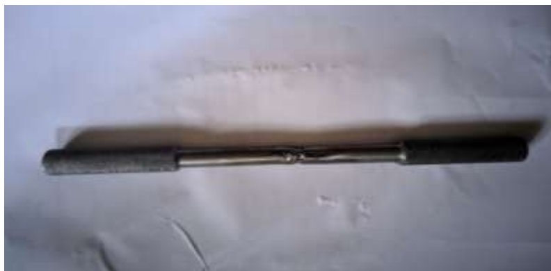
Fig. MIG weld specimen for tensile test
